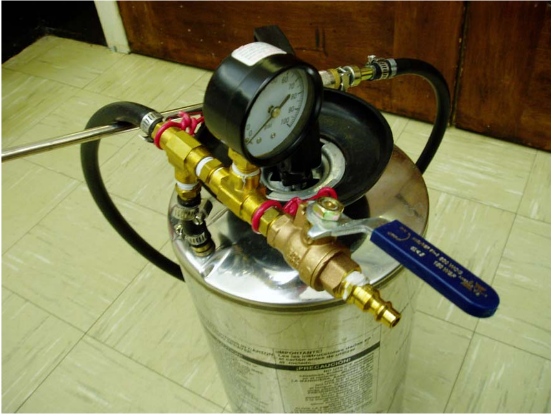
Figure 9. Close-up view of retrofitted garden sprayer
