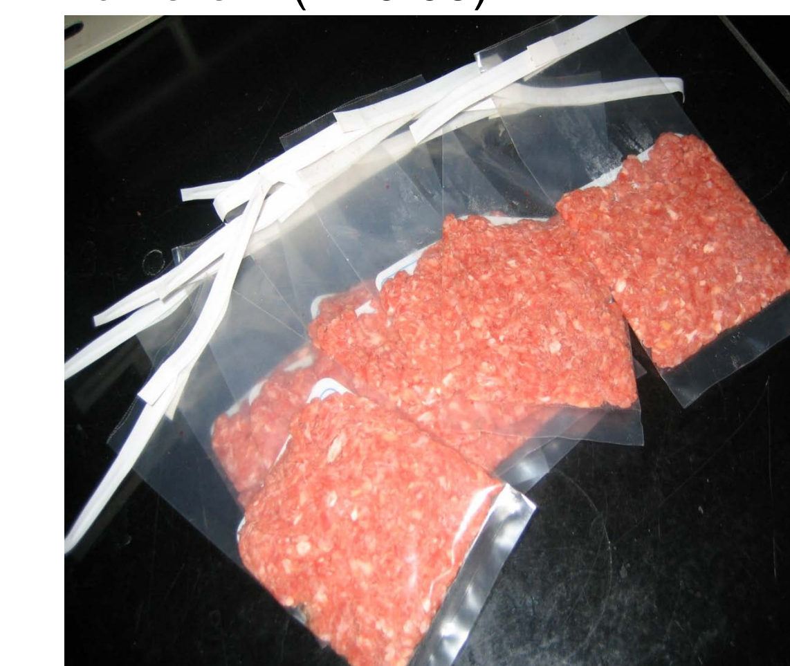
Figure 1: Small sample bags of 25g lean ground beef heated in hot water bath for heat-shock and isothermal heating experiments.
